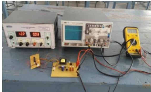
Fig. 9 Hardware implementation of SEPIC converter with 12V input
