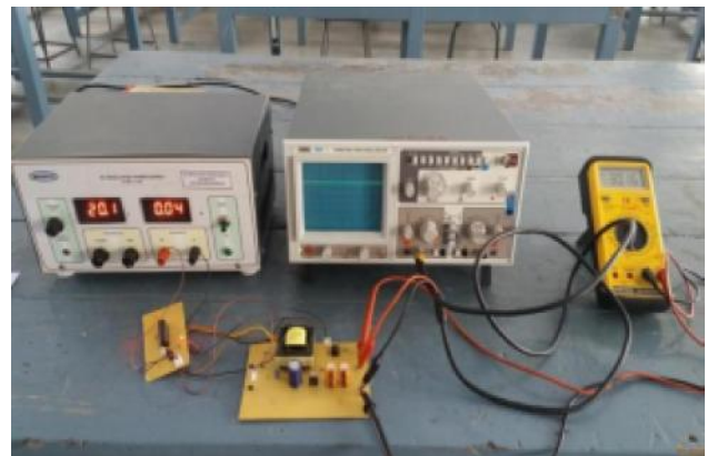
Fig.10 Hardware implementation of SEPIC converter with 20V input
