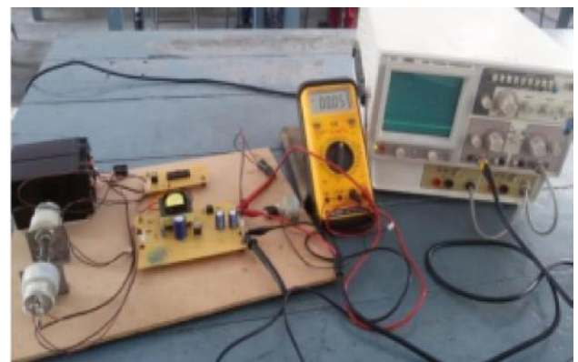
Fig.11 SEPIC converter with WECS
